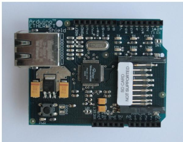
Slika 5. Arduino Ethernet Shield.
